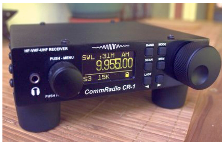
Left: Elad FDM-S2, which covers 9 kHz-52 MHz, the broadcast FM band, and 135-160 MHz. The SDR retails for around $520. (Courtesy: Elad) Right: self-contained, battery operated unit which functions basically like a standard SW radio, but which has the capability to be connected to a computer and operated like a traditional SDR. (Courtesy: CommRadio)
