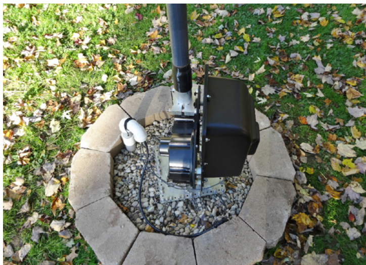
Modification of existing mounting base—originally a DXE tilt base.
