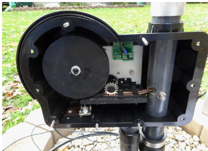
Internal detail of EHU—note tape and sprocket drive.
