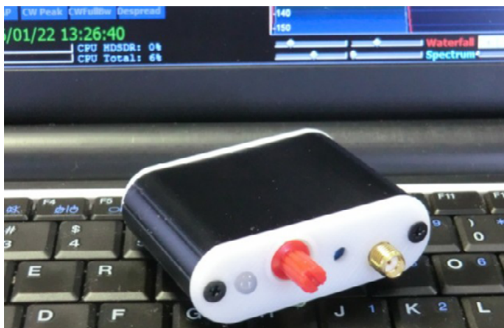
Soft66RTL3 RTL-SDR plus upconverter, plus RF amp combination circuit. (Courtesy: RTL-SDR.com)
