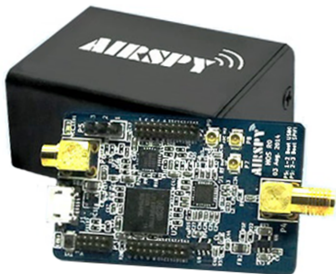
AirSpy R2 (left) and SpyVerter (right) The basic unit covers 24 MHz to 1.8 GHz, while the add-on SpyVerter takes coverage down to DC range. It has a 10 MHz view capability, which means one can see a lot of spectrum in one swipe. (Courtesy: AirSpy)
