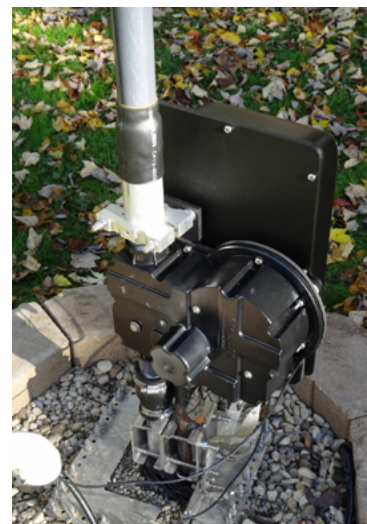
Left: Shrink tube installed at antenna joints. Center: Assembled fiberglass mast and element housing unit (EHU). Right: Installed antenna with 80 meter coil option.
