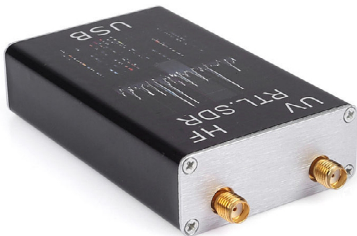
Left: Beyond the capabilities of the USB Dongle, the RTL-SDR has two antenna connectors so there is no need to swap out antennas when switching between VHF and HF. (Courtesy: Radioddity.com) Anker Astro E3 ultra-compact portable charger. (Amazon.com)
