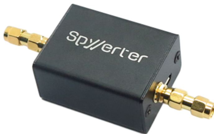
AirSpy R2 (left) and SpyVerter (right) The basic unit covers 24 MHz to 1.8 GHz, while the add-on SpyVerter takes coverage down to DC range. It has a 10 MHz view capability, which means one can see a lot of spectrum in one swipe. (Courtesy: AirSpy)
