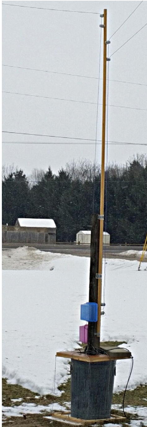
This “hastily constructed in winter” fan inverted-L vertical antenna won’t win any beauty contests and its transmit functionality to date has been merely adequate. But its receive performance is magical—but we don’t know exactly why! Perhaps you do? (NT0Z photo)
