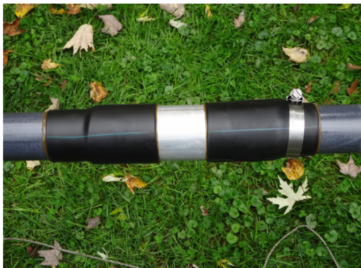
Left: Shrink tube installed at antenna joints. Center: Assembled fiberglass mast and element housing unit (EHU). Right: Installed antenna with 80 meter coil option.
