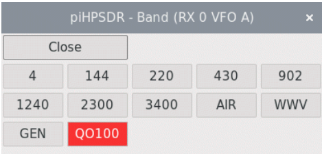
Fig. 7.9: The Band menu after defining the QO100 band.
