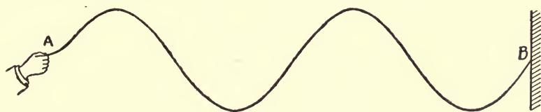
FIG. 38.—Wave motion in a rope.
