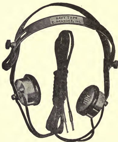
FIG. 146.—A pair of radio telephones.
