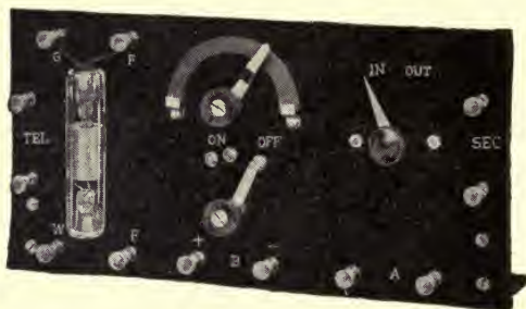
FIG. 168.—Vacuum bulb receiving set.
