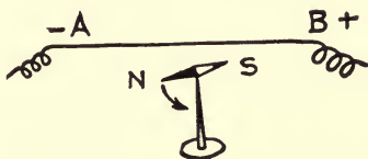
FIG. 16.—Magnetic effect of current-carrying wire.
