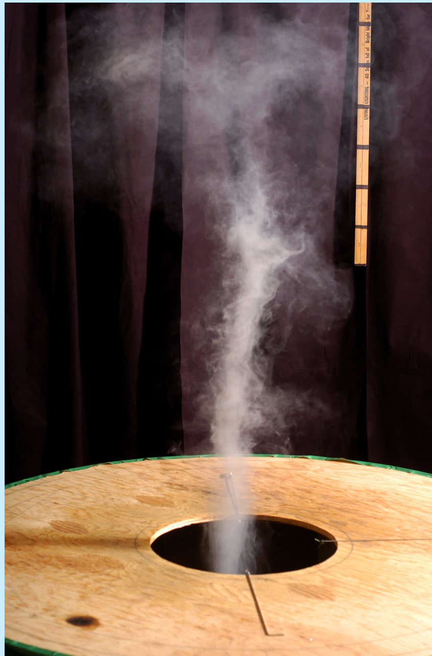
Vortex in 1 meter diameter physical model
