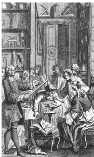
Figure B.18: Representation of Gray's famous experiment in Nollet's book, [Nol53]. In this figure it can be seen that the glass tube does not need to touch the boy.
